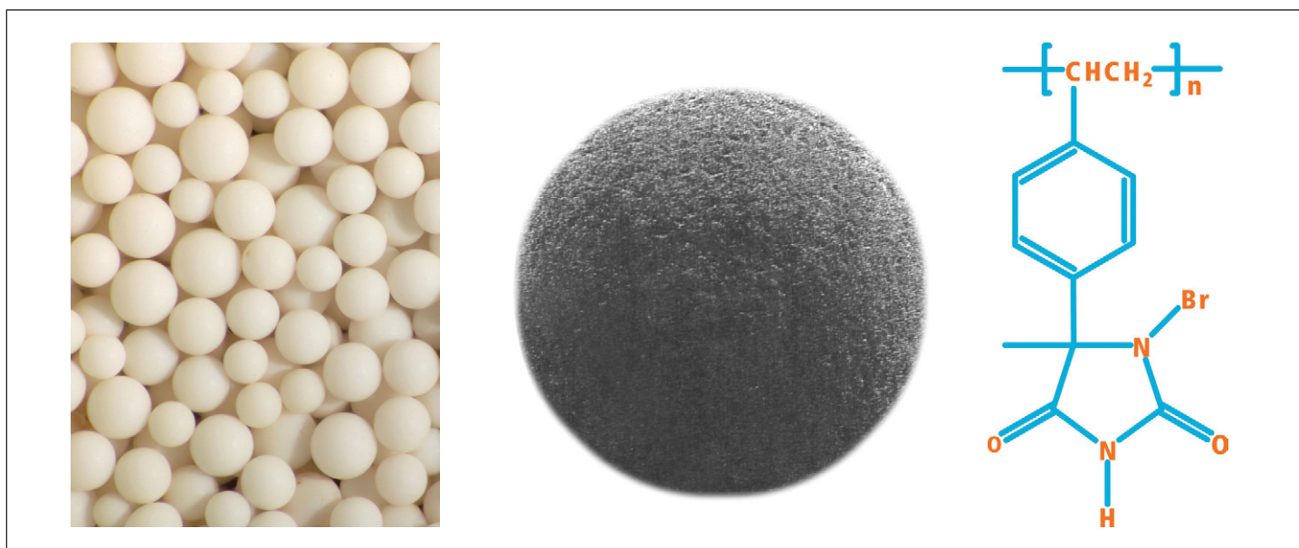
Figure 1: Porous polystyrene beads are derived by in situ synthesis of heterocyclic rings on each styrene unit that can be charged with halogen atoms (at X1, X2) to create N-halamines.
